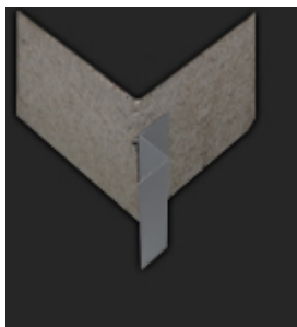
Install EcoStud on outside corner
