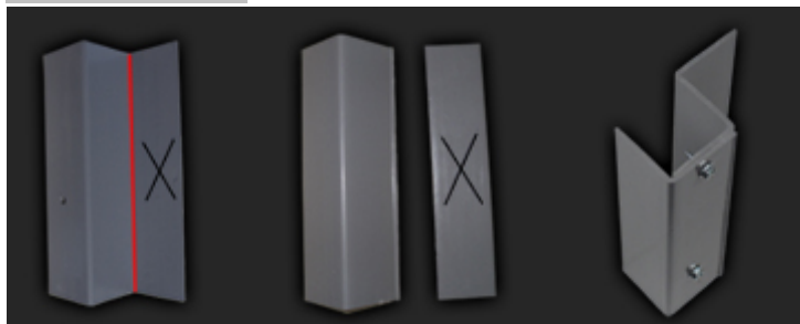
Rip EcoStud on the red line Save the piece on the left, discard right piece Attach cut piece to a full EcoStud with 1/2" needle pointed screws to create your corner bead
